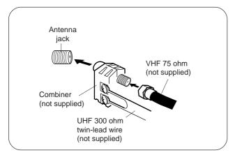
Connect the VHF 75 ohm cable and UHF 300 ohm twin-lead wire to the combiner (not supplied). Attach the combiner to the antenna jack.
